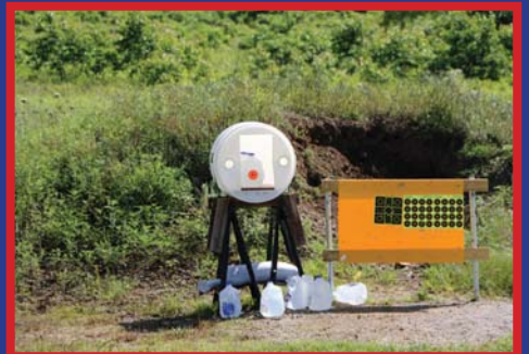
#3 A rain barrel demonstration uses a row of water jugs inside a barrel to contain any bullet fragments that result from a bullet striking the target, enabling spectators to compare ammunition and see the results firsthand.
