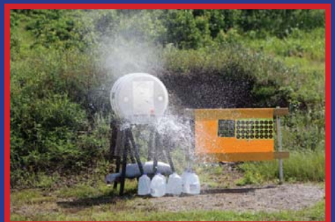
#3 A rain barrel demonstration uses a row of water jugs inside a barrel to contain any bullet fragments that result from a bullet striking the target, enabling spectators to compare ammunition and see the results firsthand.
