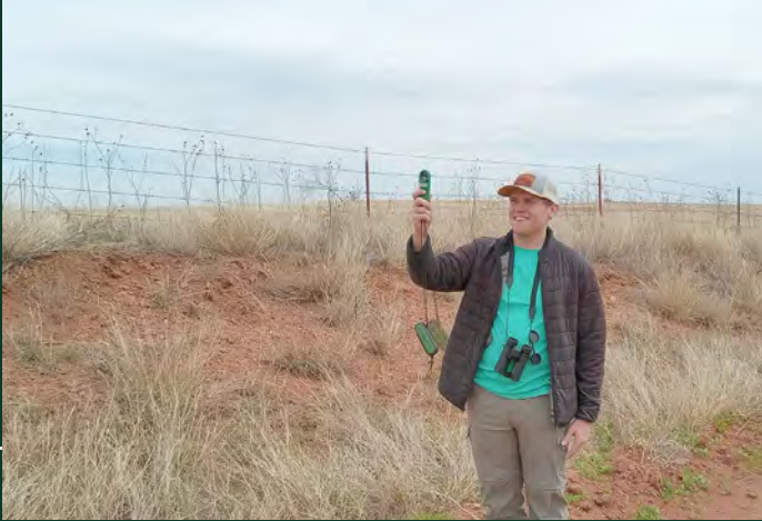
Brayden Burke measures wind speed as surveying cannot be performed if above 12 mph Photo by Kendall Van Zanten
